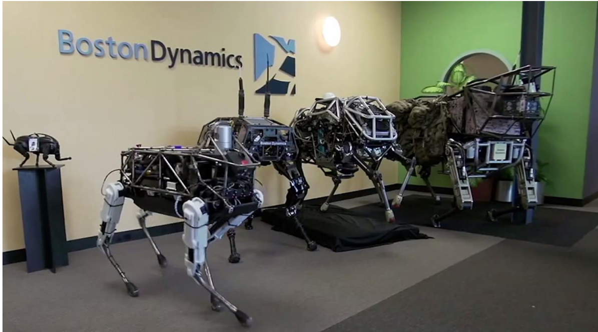
Figure 2-4: Quadruped Robots from Boston Dynamics: LittleDog, Spotmini, Cheetah robot and BigDog
