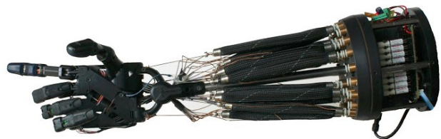
Fig. 2: Robotic hand using air muscles, image credit Shadow Robot Company [26]
