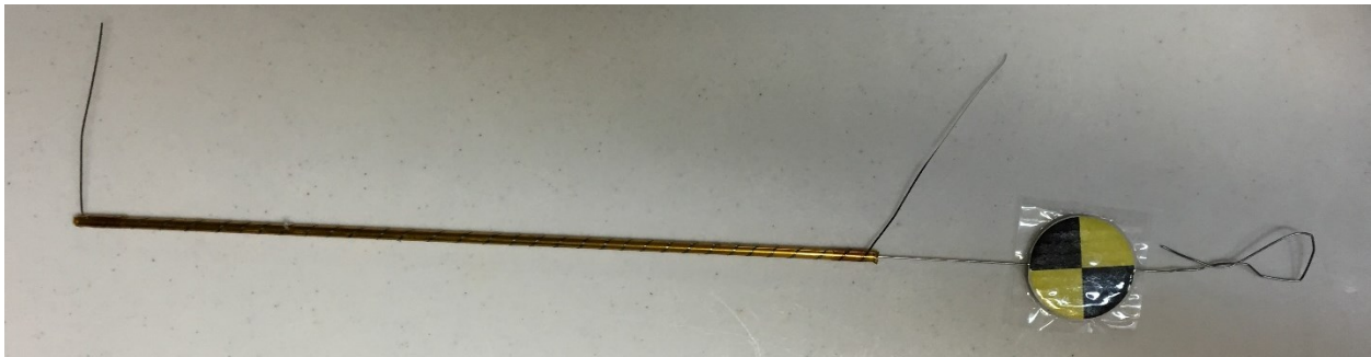
Fig. 7: Heater Tube and Hanger System
