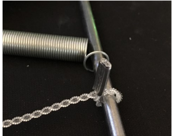
Fig. 8: Steel Pin with Attached Muscle and Spring
