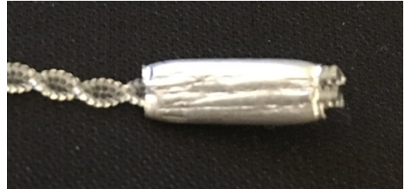
Fig. 5: Crimped aluminum tube on end of two-ply muscle
